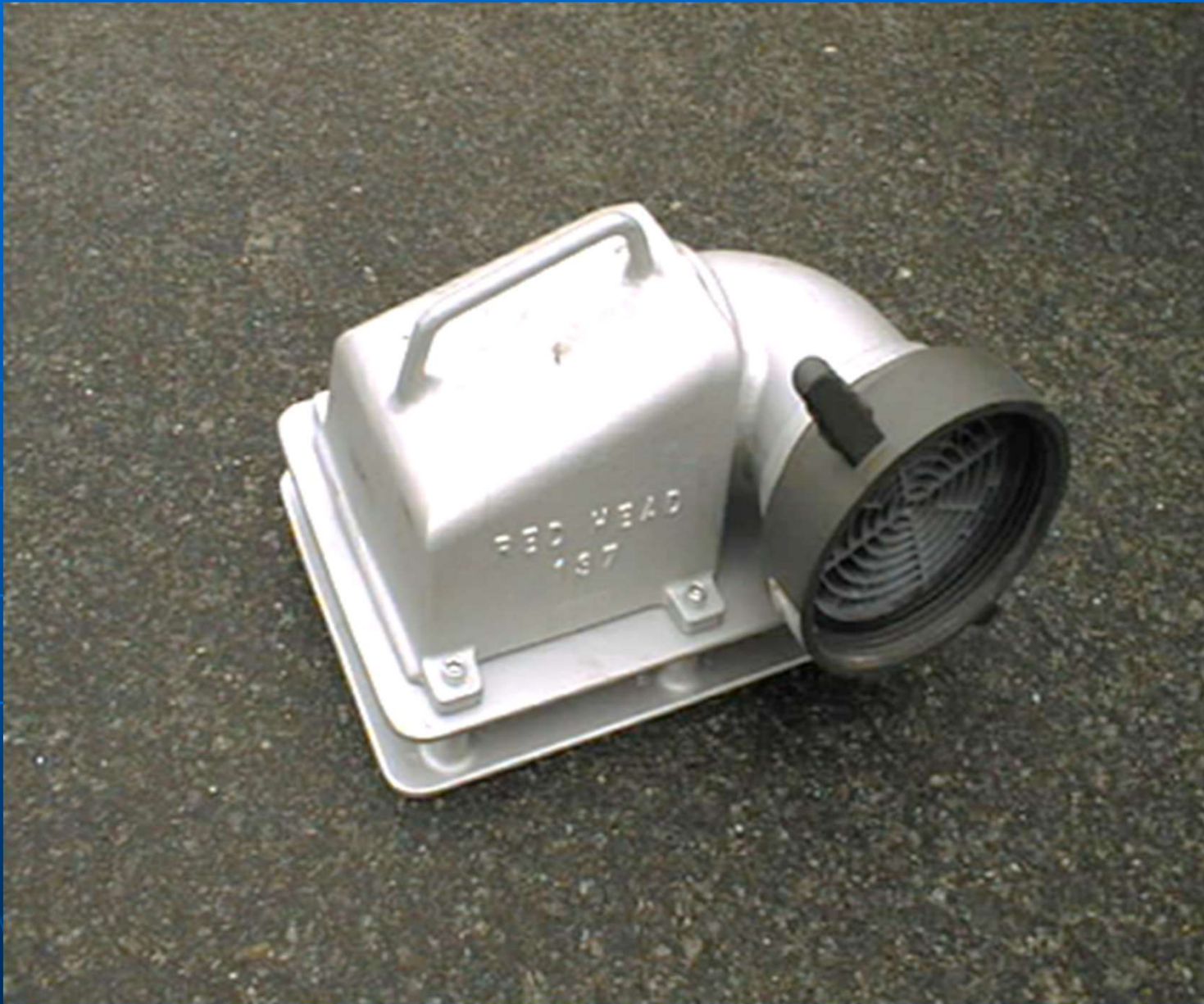
Low Level Strainer: For drafting from Drop Tanks.
